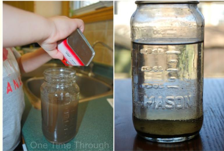
After three hours, you should return to find the Alum mixture has settled to the bottom of the jar.
