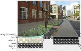
Concrete Transition Strip pervious congrete (min 6\*) structural layer (min 6\*) Hydraulic Restriction Layer Geotextile (as required)
